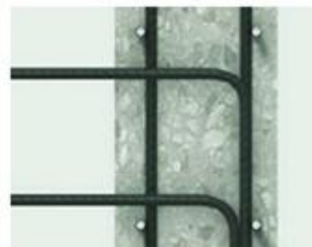
Traditional slab-to-wall construction joint Drilling of formwork required, projecting reinforcing bars and congestion in the wall.
