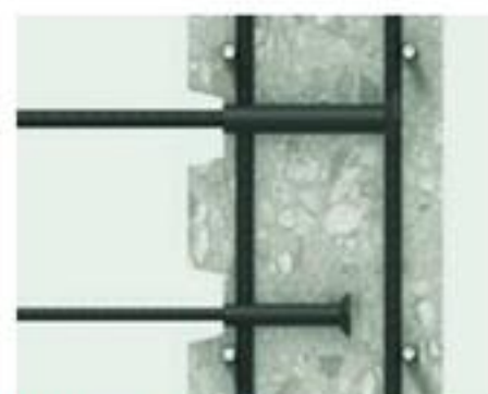
NEW high performance, KSN Anchor system Anchors installed in a carrier. Indented construction joint. Virtually unlimited bar length. No bending of bars required. Less congestion in the wall.
