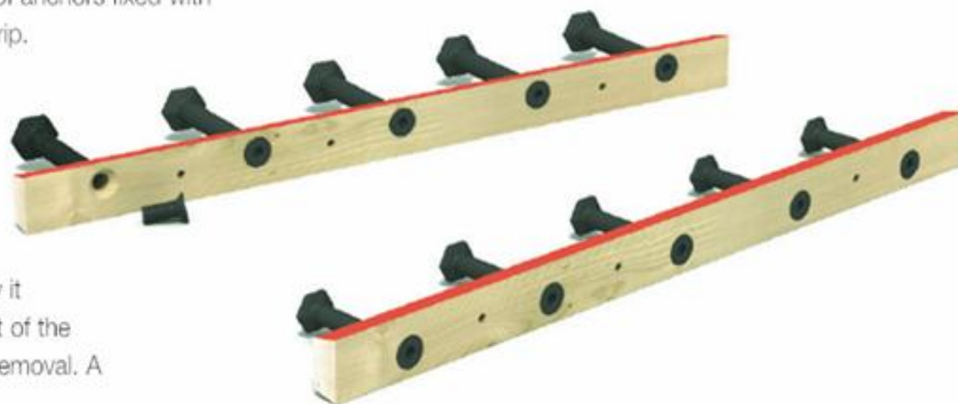
Tapered timber strips simplify installation, create a shear key and increase anchor embedment
