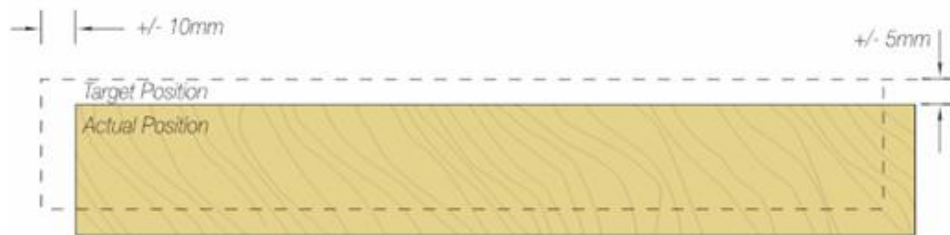
Timber Anchor Carrier Setting Out Deviation Allowances
