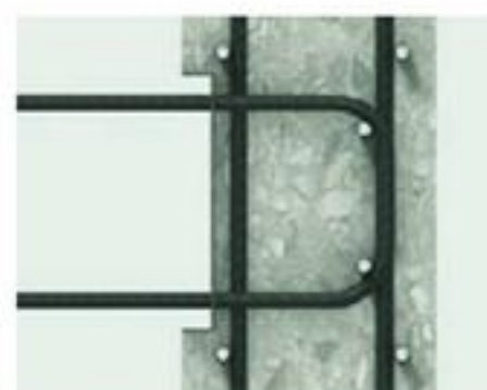
Re-bend continuity system Box dimensions restrict bar length and diameter. On-site bar straightening required.
