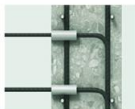
Reinforcing bar couplers Awkward anchorage bars. Congestion in the wall. No shear key. Individual coupler installation slows site progress.
