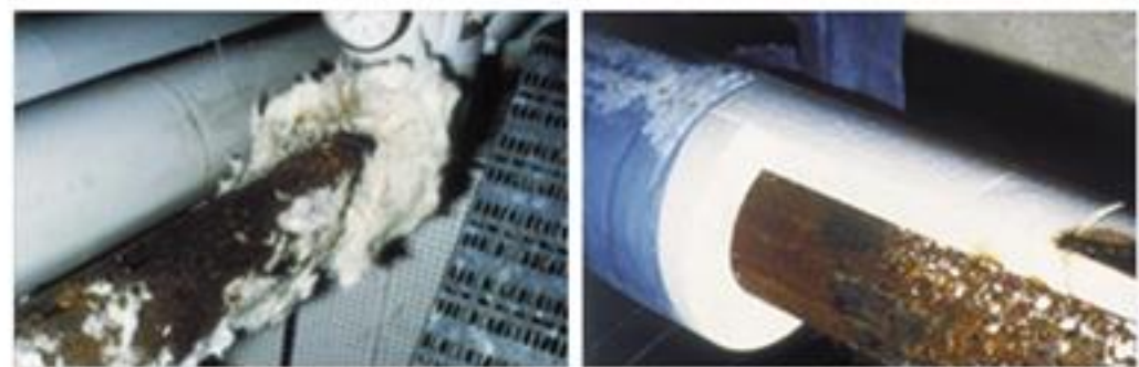
The consequences of choosing the wrong insulation for cold systems can be serious and costly.
