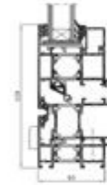
Pivot window - cross section
